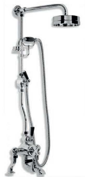
MK 8825 MACKINTOSH THERMOSTATIC BATH SHOWER MIXER WITH RISER KIT, HANDSET, LEVER DIVERTER, 8" ROSE & ADJUSTABLE RISER PIPE BRACKET
